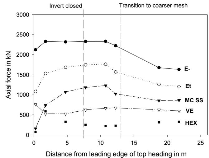
Figure 6: Axial forces in tunnel lining at crown
