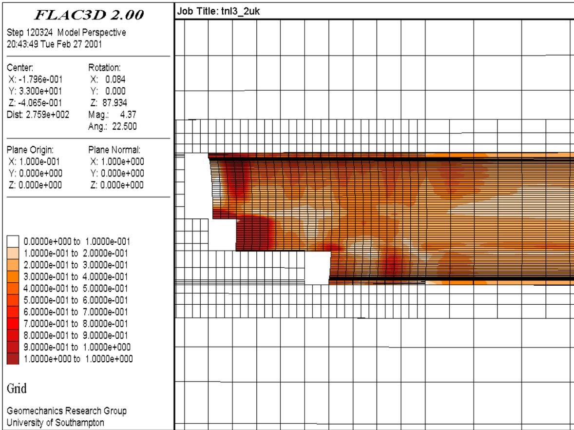
Figure 8: Utilization factors for elastoplastic SCL model (MCSS).
