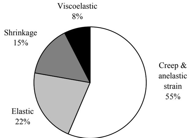
Figure 2. Composition of strains after 240 hours for SFRS under uniaxial compression (after Ding 1998)
