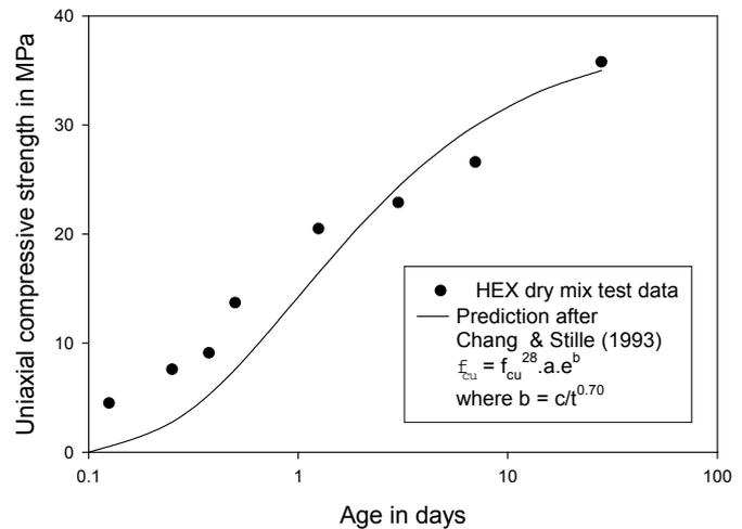
Figure 3: Strength gain of sprayed concrete, with data from Heathrow Express Project
