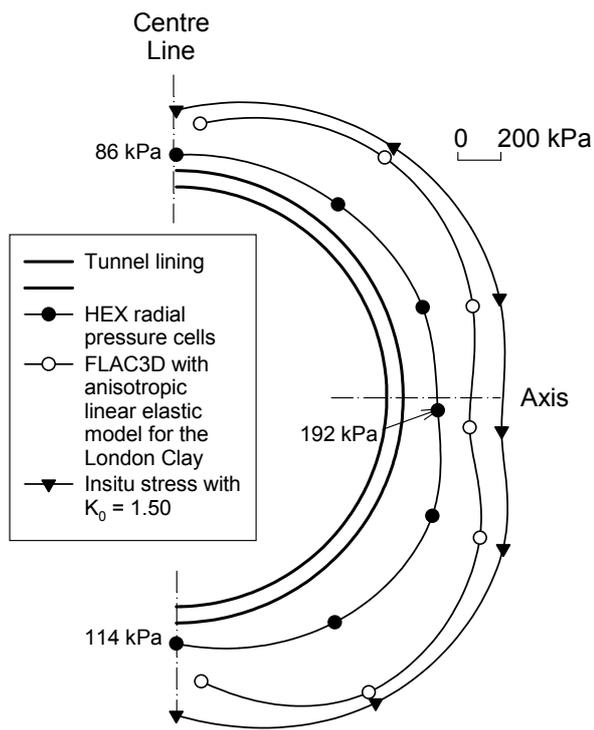
Figure 5: Radial stresses acting on tunnel lining
