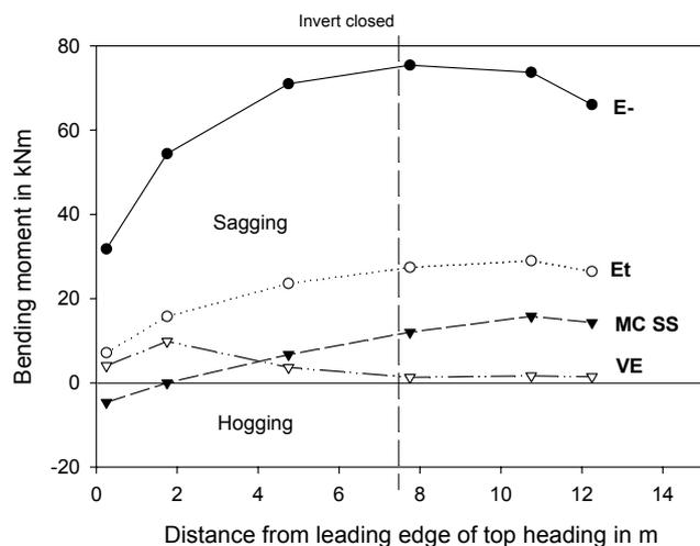
Figure 7: Bending moments in circumferential direction at crown
