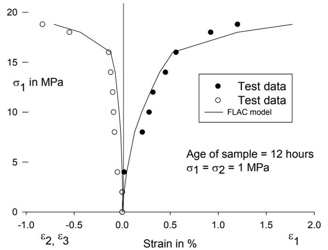
Figure 1. Behaviour of spray concrete under triaxial compression (Brite Euram 1997) with predictions using Kotsovos & Newman nonlinear elastic model in FLAC3D.
