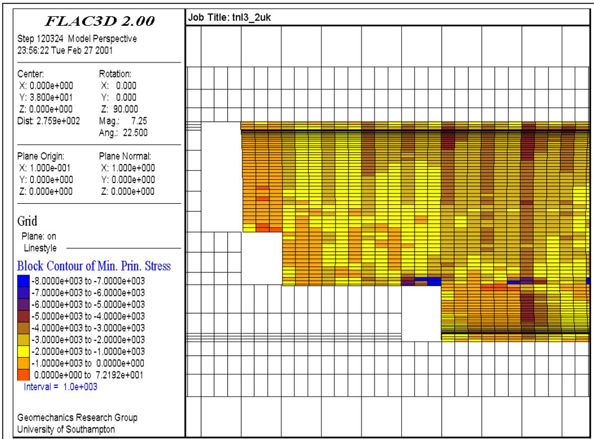
Figure 9: Circumferential stress in the tunnel lining for the elastoplastic SCL model (MCSS).
