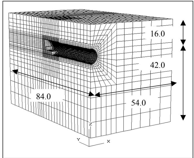
Figure 4: FLAC3D model for HEX platform tunnel
