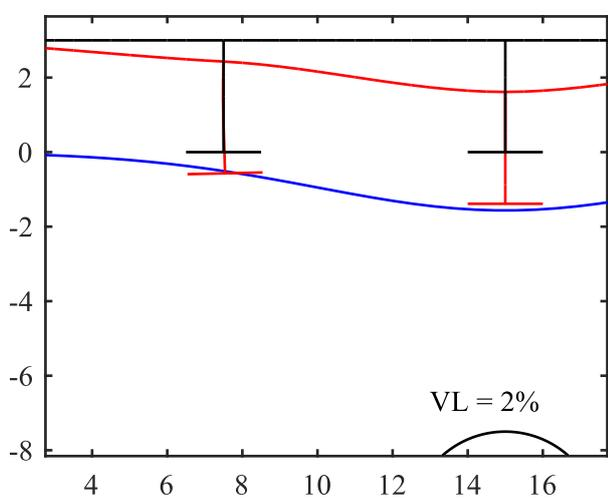
Figure 8. Deformed shape showing footing rotation in opposite direction to greenfield profile (displacements ×50 times)
