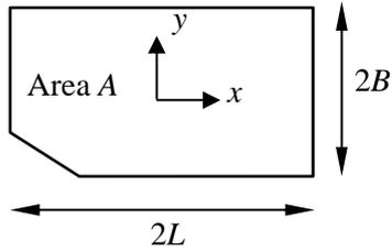
Figure 3. Definition of dimensions and reference axes for footing of arbitrary shape after Gazetas (1991),  $x$  and  $y$  axes being the minor and major principal axes respectively for the circumscribed rectangle
