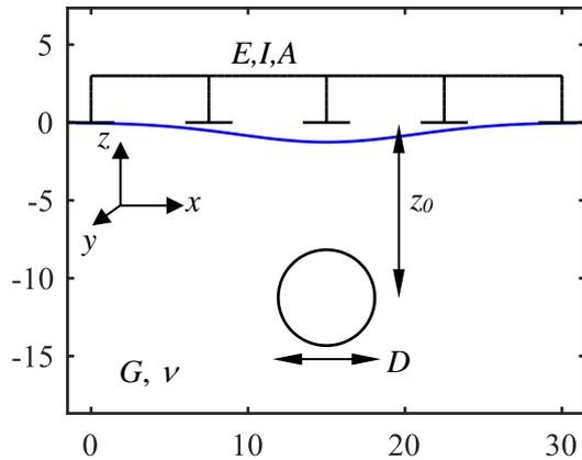
Figure 2. Plane frame on rigid footings founded on elastic half-space
