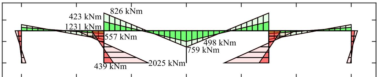
Figure 5. Bending moments for deformed frame (i) under imposed greenfield movements (light colours)  $M_{gf}$  and (ii) considering soil-structure interaction (dark colours)  $M_{ss}$
