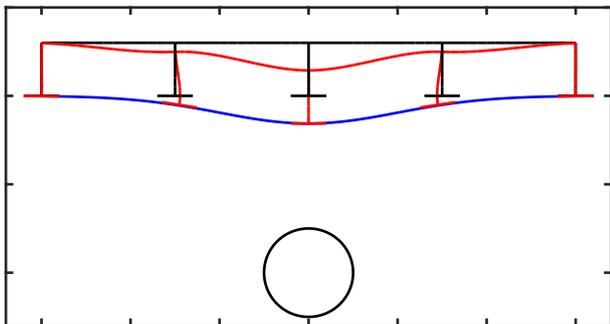
Figure 1. Displacement of a framed structure (red) following greenfield settlement profile (blue)
