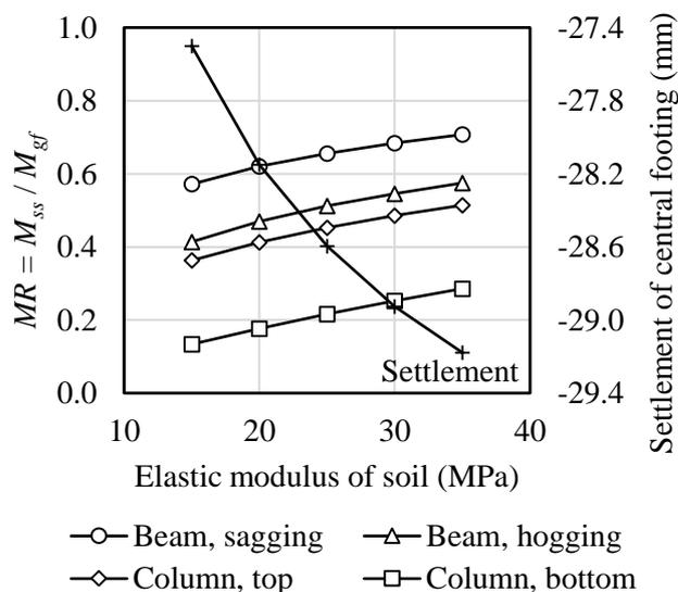
Figure 9. Effect of elastic modulus of founding soil on bending moment and settlement
