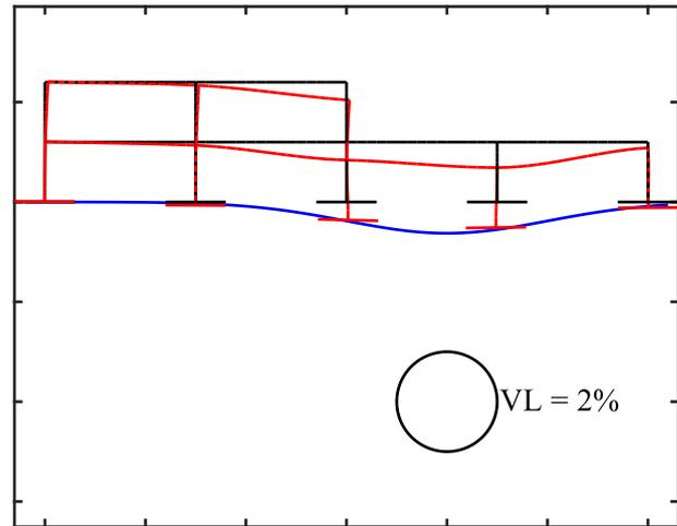
Figure 10. Deformation of two-storey framed structure
