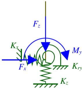
Figure 4. A column connected to a rigid footing represented by foundation springs  $[K_f]$  (green) and subjected to equivalent tunnelling forces  $\{F\}$  (blue)
